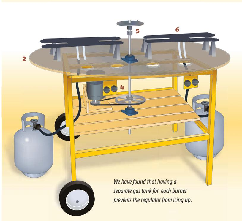
*We have found that having a separate gas tank for each burner prevents the regulator from icing up.*
